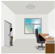
With ambient light more than daylight threshold, the lamp does not switch on when someone enters the room
