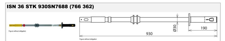
Insulating stick IS 36 STK. With plug-in coupling at both ends for attaching extension elements, operating heads or adapters. Single part of insulating stick kit IS STK.
