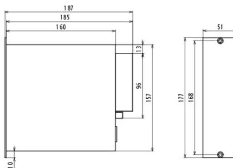
DSRT DD FS .... detection device for light detection (DSRT FS fibre optic sensor).
