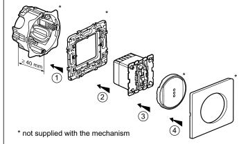
2 - The rocker is clipped to the mechanism.
