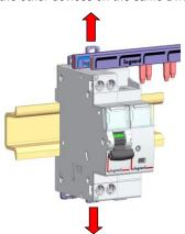
1. Unclip the clamp to put it in open position
