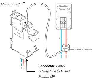
Wire the Connected energy meter after a circuit breaker. The connection between the energy meter and the coil is made via a locking connector.
