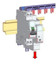
3. Pull the device downward in order to completely release it from the prongs of the busbar
